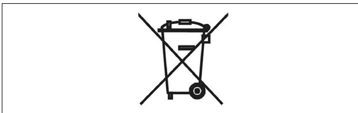
Figure A1-2: Symbol for the marking of EEE (it must be printed visibly, legibly and indelibly)
